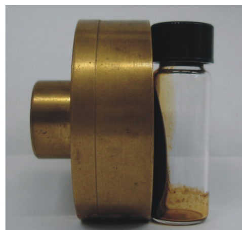
Figure 14. Encapsulated taxol and MF-PEG in PLGA attached to a magnet.
